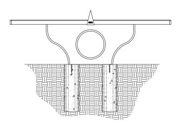
For zones subject to freezing, HENGE recommends concrete reinforced footer placement using 12" sonotubes or similar.
